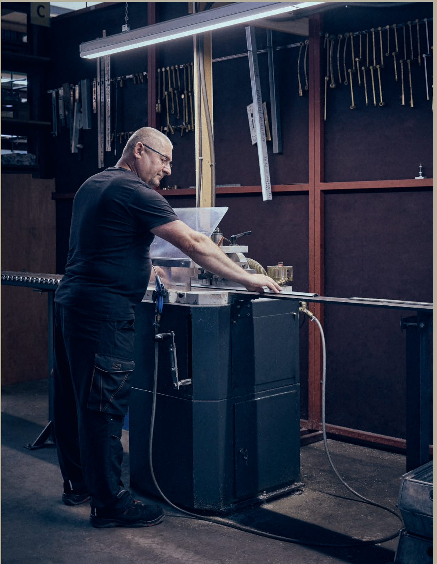
Cutting of aluminum profiles. The image shows the Epsilon profile .
